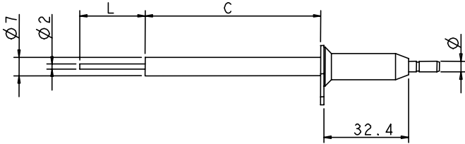
Fig. 3 Electrode with teflon cable and resistor
