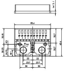
(\*) The dimensions differ according to the type of socket: 5 with socket A 9 with socket B
